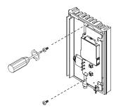
Reinstall the faceplate on the base and secure it in place with the screw.
